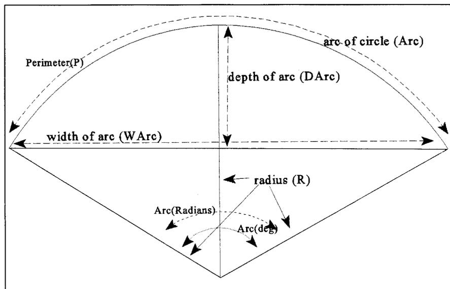
Figure 2. Diagrammatic representation of depth and width of arc.
